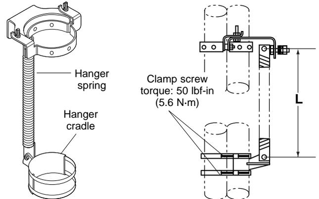
**Vertical Spring Hanger Spring Settings - L, in (mm)**
