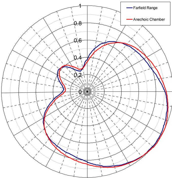
Figure 2: CH32 Azimuth Pattern Comparison
