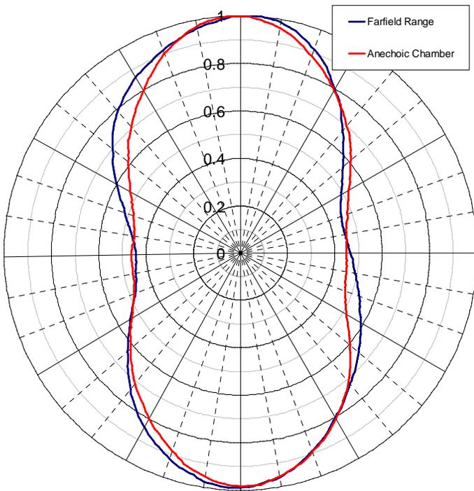
Figure 3: CH26 Azimuth Pattern Comparison
